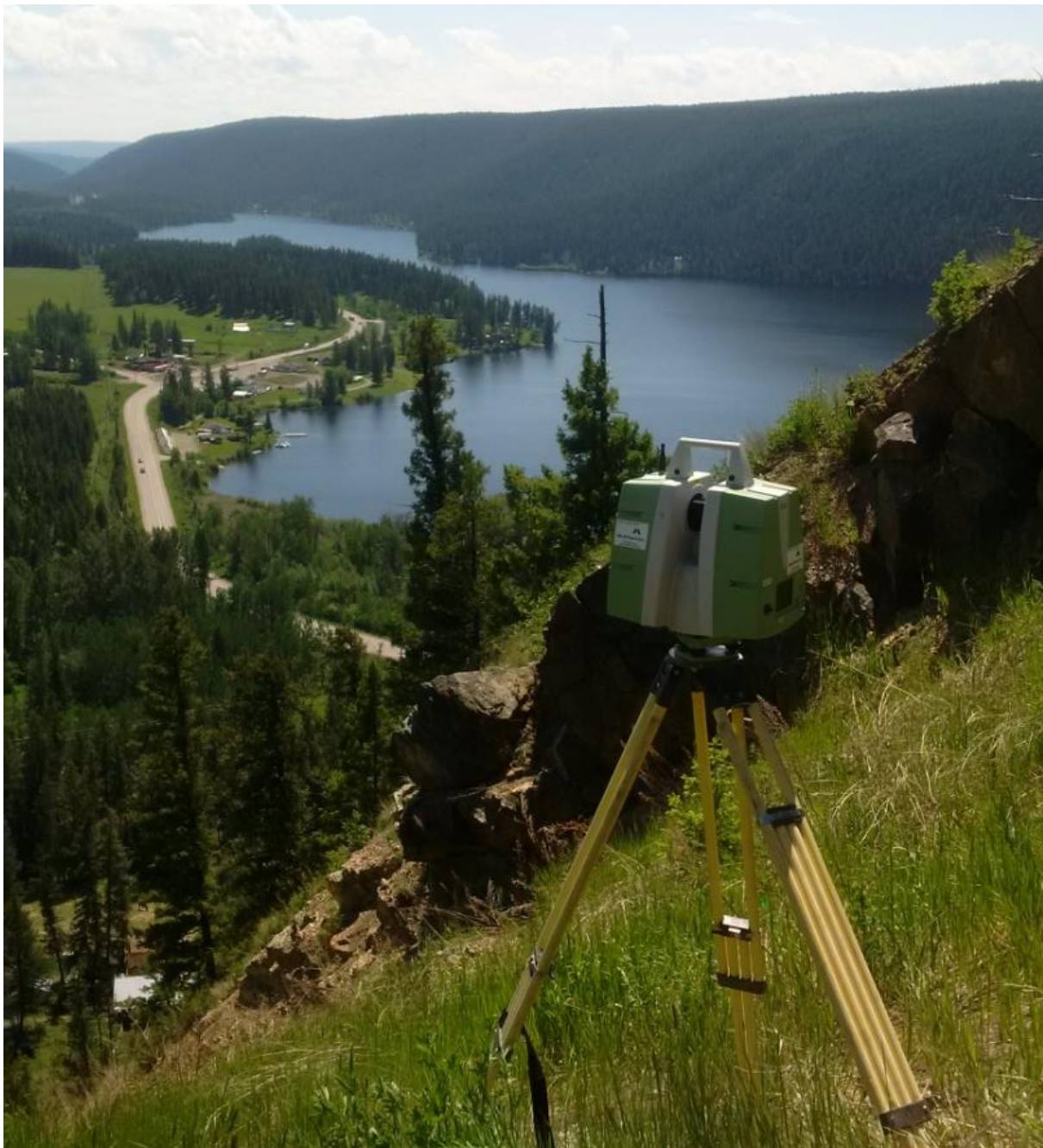
Figure 8-59 Looking north from top of a pipeline ROW slope where a blasted rock slope is a source of rock falls onto the ROW and a deeper translational slide is forming. Device is a mid-range panoramic scanner. (Photo by: S. Boon, Year: May 2015)
