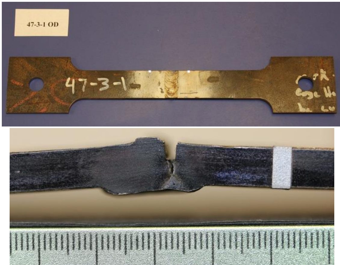
Figure 5-94 Top view and side view of artificial flaw CWT specimen partially broken in weld
