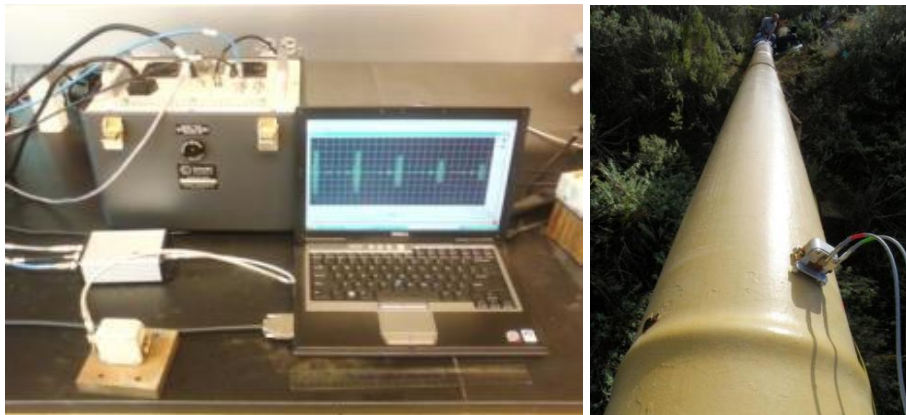
Figure E-33 Prototype Strain Measurement System and EMAT probe
