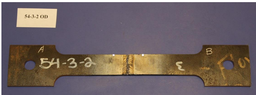
Figure 5-93 Artificial flaw CWT specimen completely broken in weld
