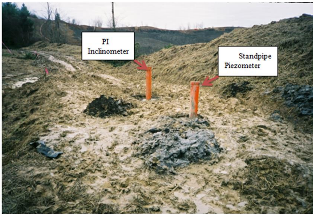
Figure 8-44 Above-ground, protective surface completions in a landslide, on a ROW, for a standpipe piezometer and a PI inclinometer (Photo by: D. West, Year: 2005)
