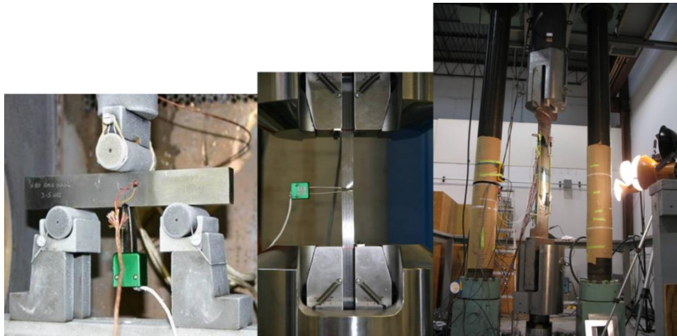
Figure 7-9 Images of various toughness test options that may provide input to the PRCI-CRES tensile strain models. Left: standard three-point bend CTOD; Middle: SENT; and Right: CWP
