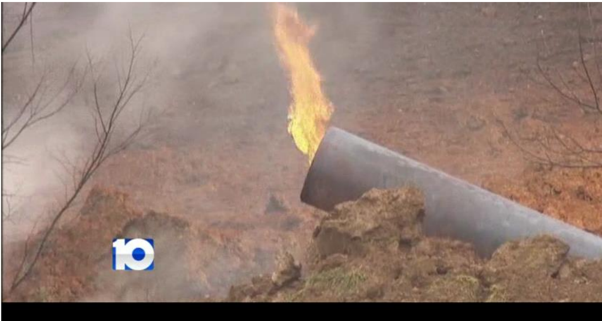
Figure 1-1 Girth weld tensile rupture and the resulting fire from a TV news report
