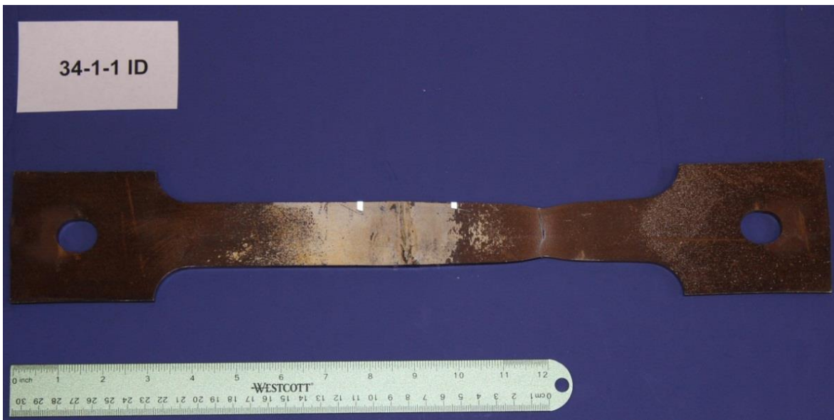
Figure 5-83 CWT specimen 34-1-1 with natural flaw failed in the base metal
