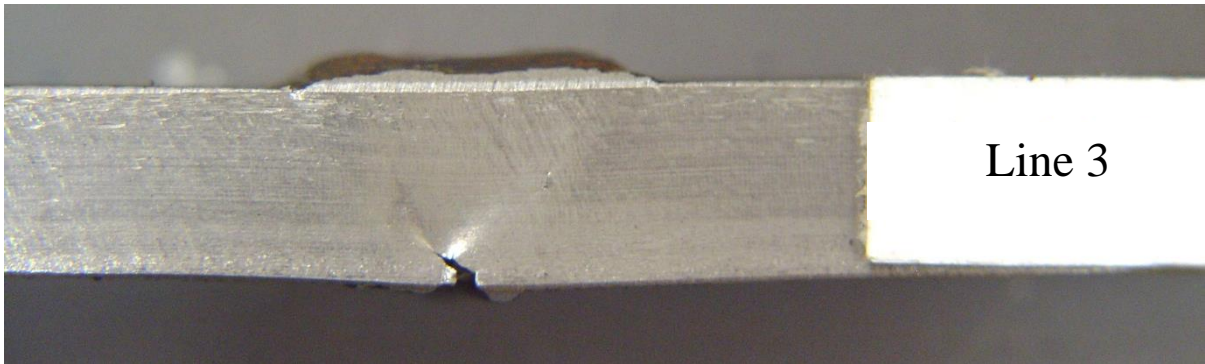
Figure 5-39 Weld cracking observed after the test of Specimen from Line 3
