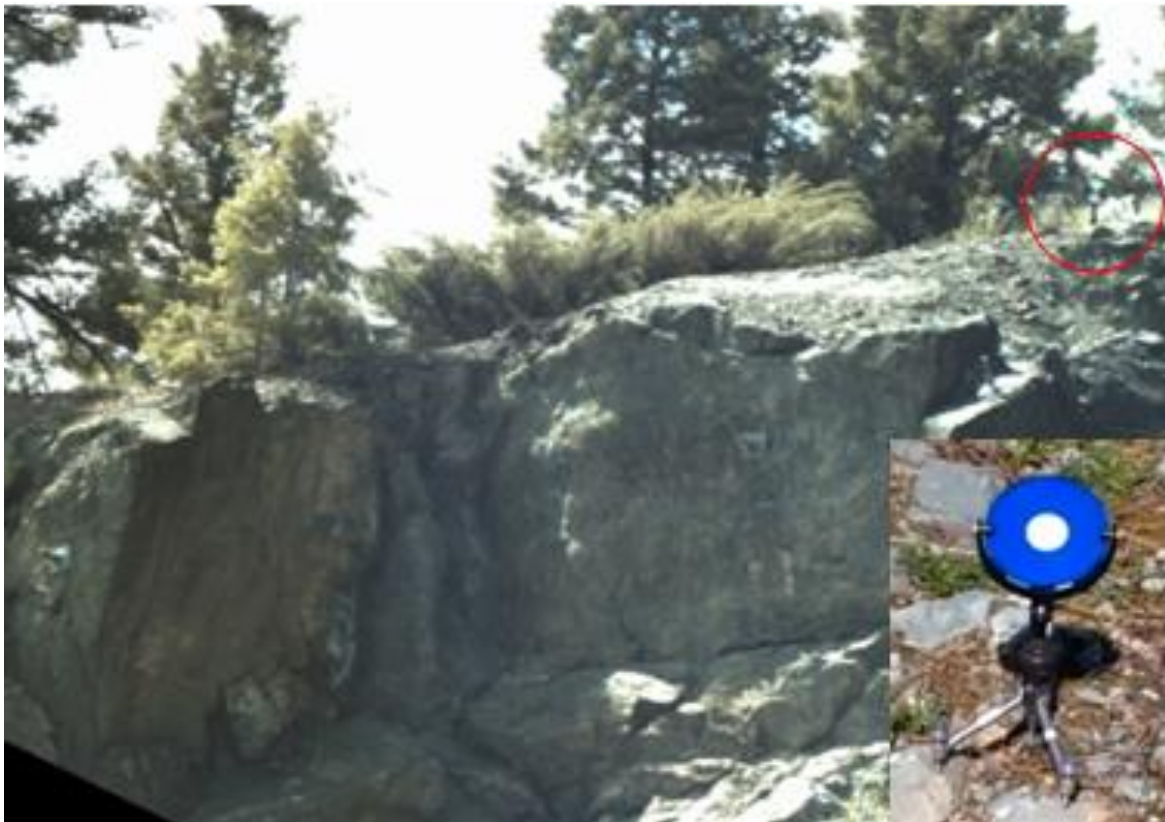
Figure 8-61 Scanned target on a control point at top of rock slope with inset showing a typical scanning target (Photo by: S. Boon, Year: May 2015)
