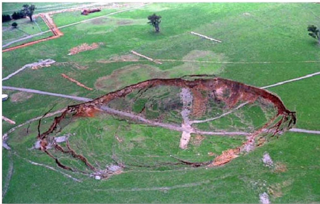
Figure 2-3 Illustration of location and types of surface subsidence deformation above a collapsed underground room-and-pillar coal mine (modified from [41]).
