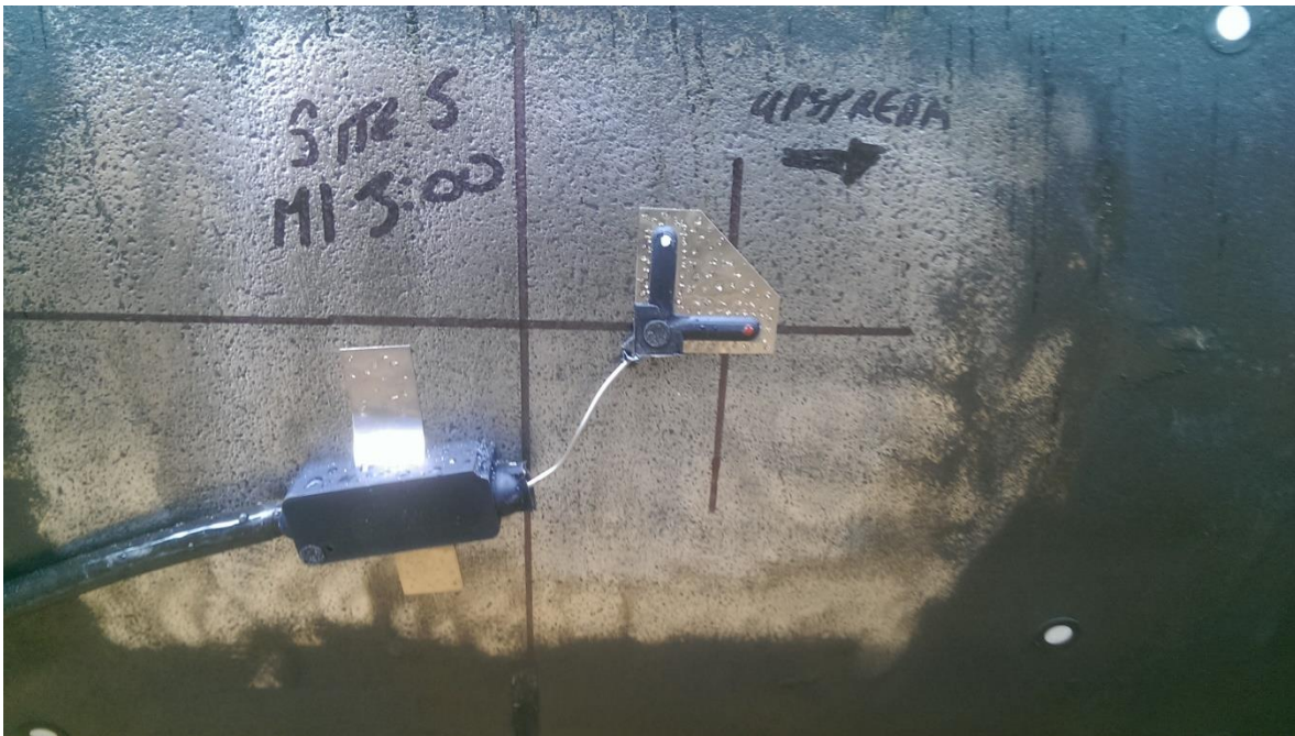
Figure 8-78 Resistance type strain gauges installed on a pipeline
