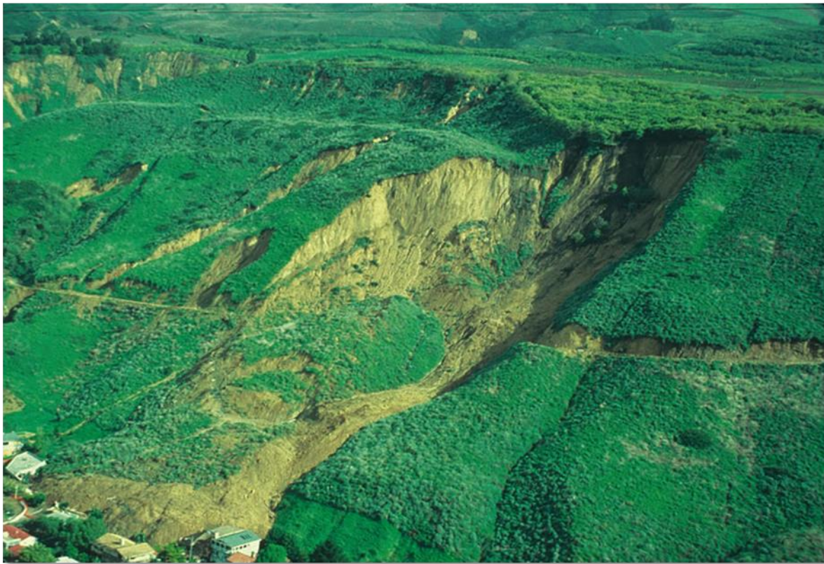
Figure 2-18 The 1995 La Conchita complex rotational earth/debris slide-earth flow in (Photo by: R.L. Schuster, USGS, Location: California, Year: 1995)
