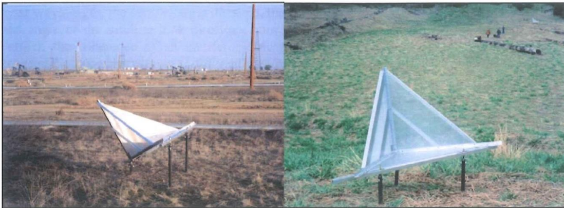
Figure 8-65 InSAR radar reflectors [7]. Note that the technology has developed to the point that over time these radar reflectors are becoming smaller and therefore more economical to install.
