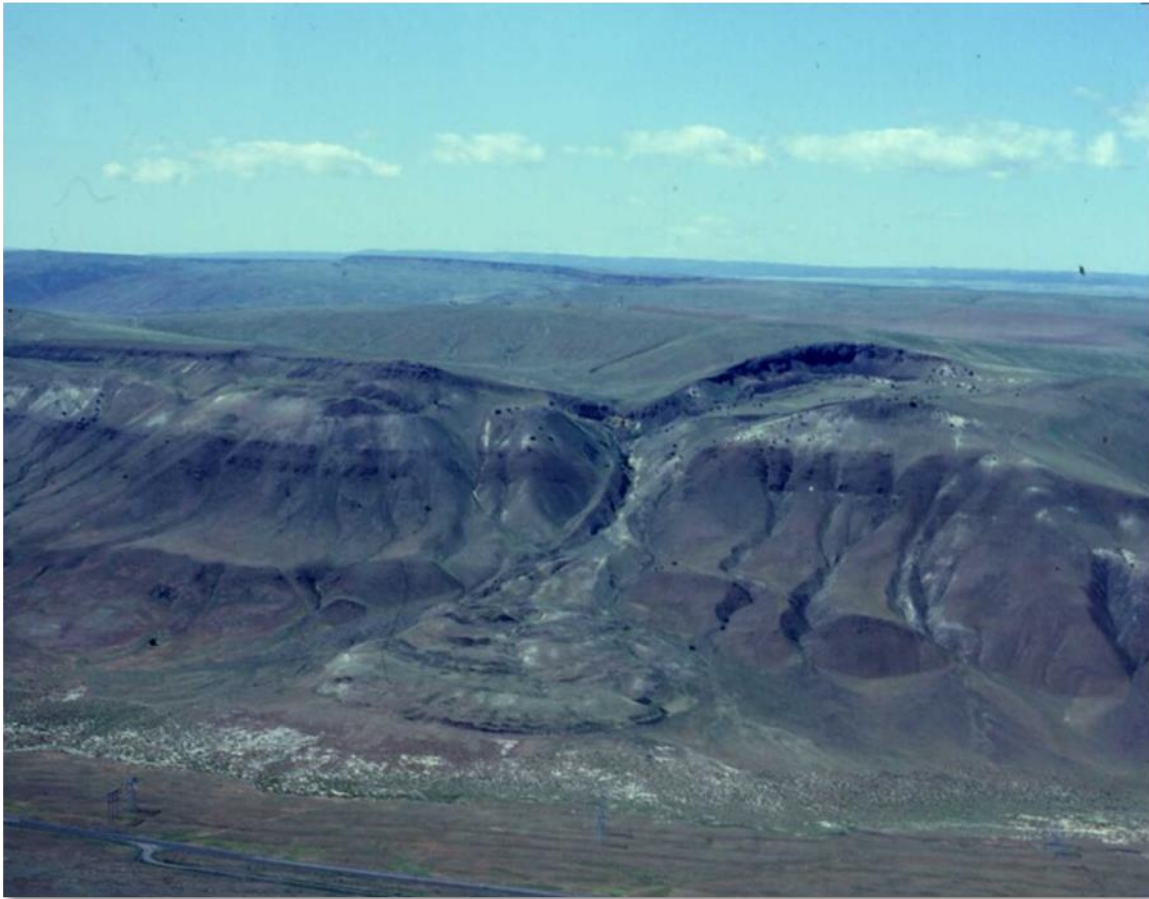
Figure 2-22 Earth flow along the Columbia River in Washington; the landslide occurred along a weak sedimentary interbed in the nearly horizontal Columbia River basalt and flowed through a drainage channel to spread out downslope. (Photo by: D. West, Year: 1995)
