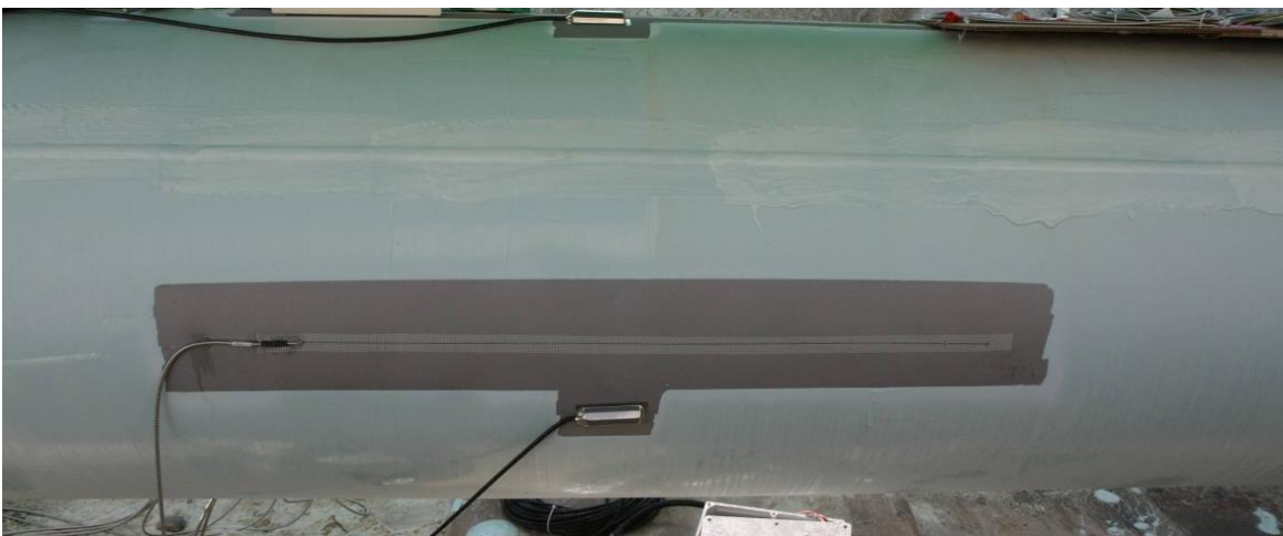
Figure 8-87 Adjacent FO and VW strain gauge installations to show size limitations of VW strain gauge size. The VW strain gauges are used to back up the FO strain gauge install in this application. (Photo by: D. Dewar, Year: 2008)
