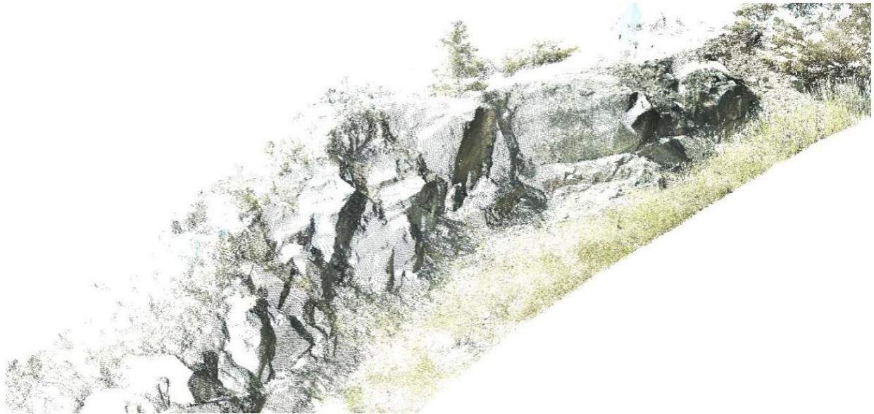
Figure 8-60 Surface model of the rock slope in the previous figure based on the point cloud produced by the survey of the slope (Photo by: S. Boon, Year: May 2015)
