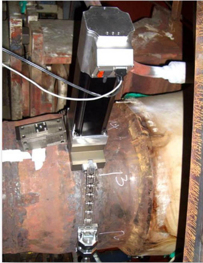
Figure E-20 Example of the application of IIT on a pipe to determine residual stress [281]
