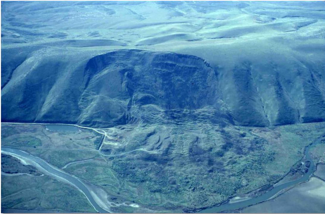
Figure 2-15 Example of an ancient translational rock slide on a steep slope in dipping, bedded basalt bedrock in eastern Washington and which transitioned into a rock/debris avalanche/flow (Photo by: D. West, Year: 1977).
