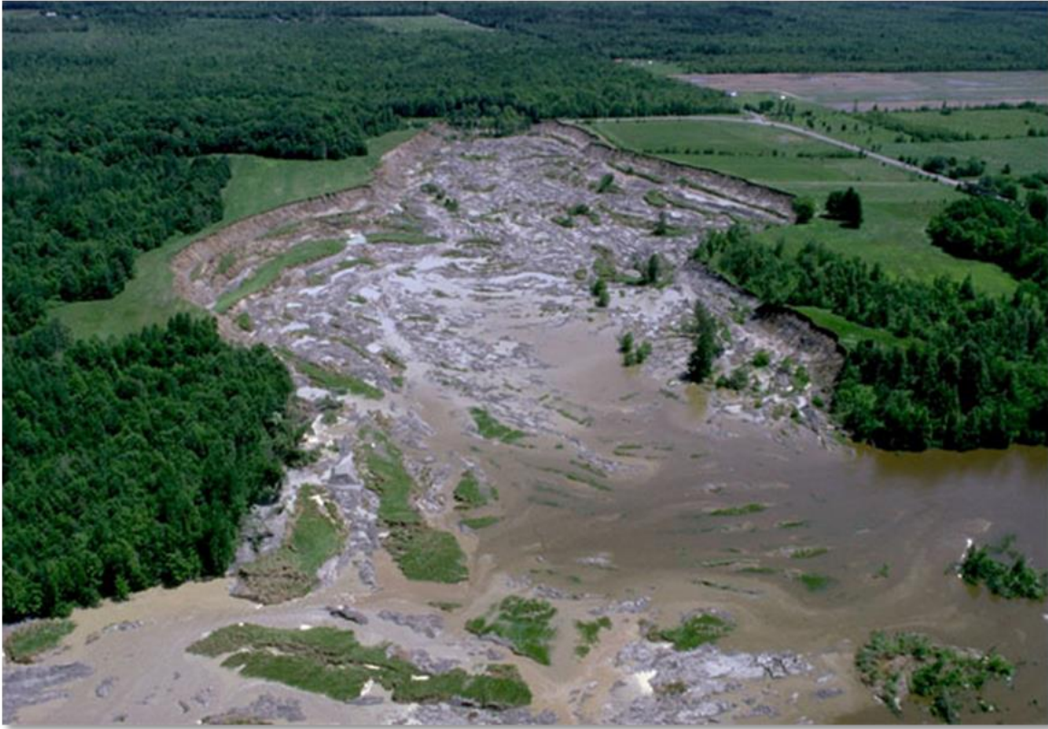
Figure 2-28 The 1993 Lemieux Slide near Ottawa, Ontario. A rapid retrogressive lateral spread triggered by liquefaction of sensitive marine clays. [63]
