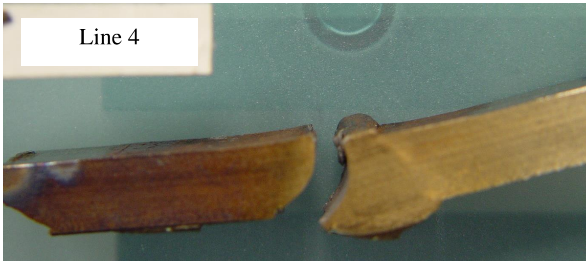
Figure 5-42 Girth weld from Line 4 was fractured in liquid nitrogen after cross-weld tensile test, showing the fracture path along the fusion line/HAZ
