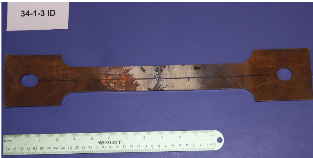
Figure 5-81 A CWT specimen with natural flaw failed in the weld region.
