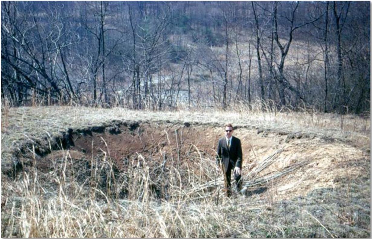
Figure 2-42 Surface subsidence pit above a coal mine (Source: S. English, Location: Harrison County, West Virginia, Year: 1970)
