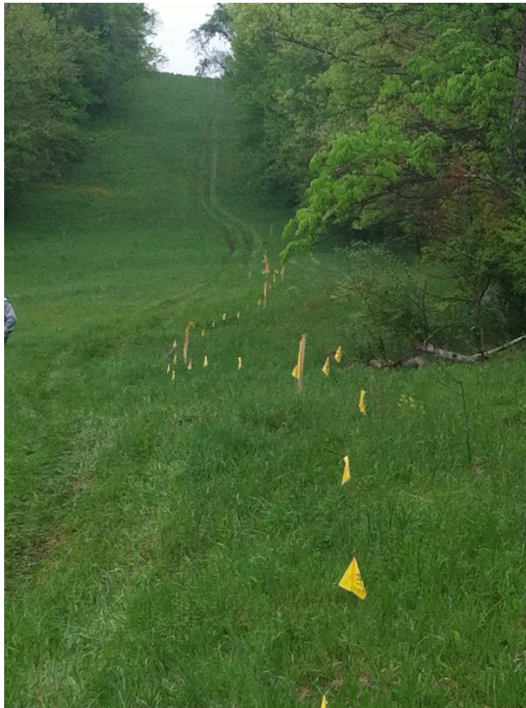
Figure 8-31 View of a line of pipeline locates (wands) through an active landslide. The landslide had deflected the pipeline laterally downslope and to the left by about 5 ft (1.5 m), maximum. The total length of pipeline deflection was about 150 ft (46 m). (Photo by: B. Albert, Year: 2013)
