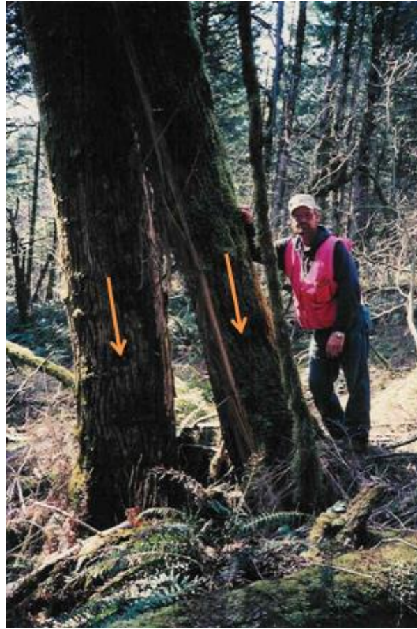
Figure 8-30 View of tilted and split tree in a landslide mass. Continued, periodic measurement of the angle of the tilt and width of the split can provide information on landslide movement. The arrows on the tree represent possible reference markers attached to the tree to aid in the successive measurement of tilt. (Photo by: D. West, Year: 1999)
