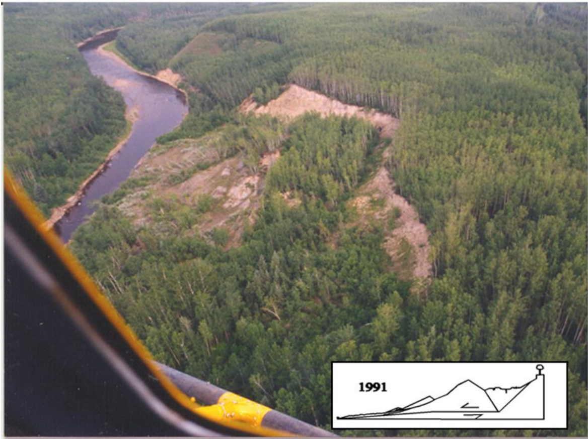
Figure 2-16 Deep seated very slow translational earth slide in Cretaceous clay shale bedrock in the McKay River Valley, northeastern Alberta. The inset is a schematic cross-section through the slide (Photo by: D. Dewar, Year: 1996).
