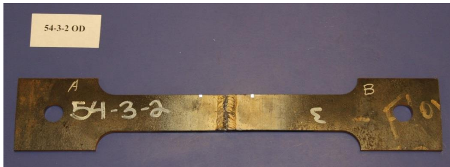
Figure 5-86 Artificial flaw CWT specimen completely broken in weld
