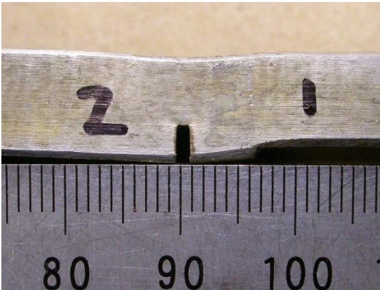
Figure 5-47 Side view of specimen Line 4-1-4a at the termination of the test
